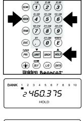
Press (10) to lockout the channel. L/O appears in display.
